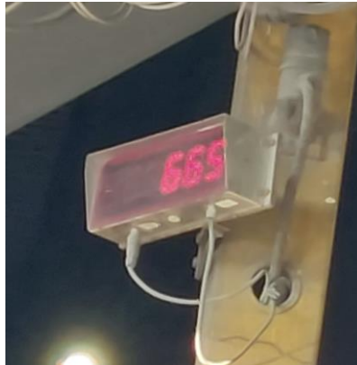
Figure 32: Weight sensor output on LED display.
