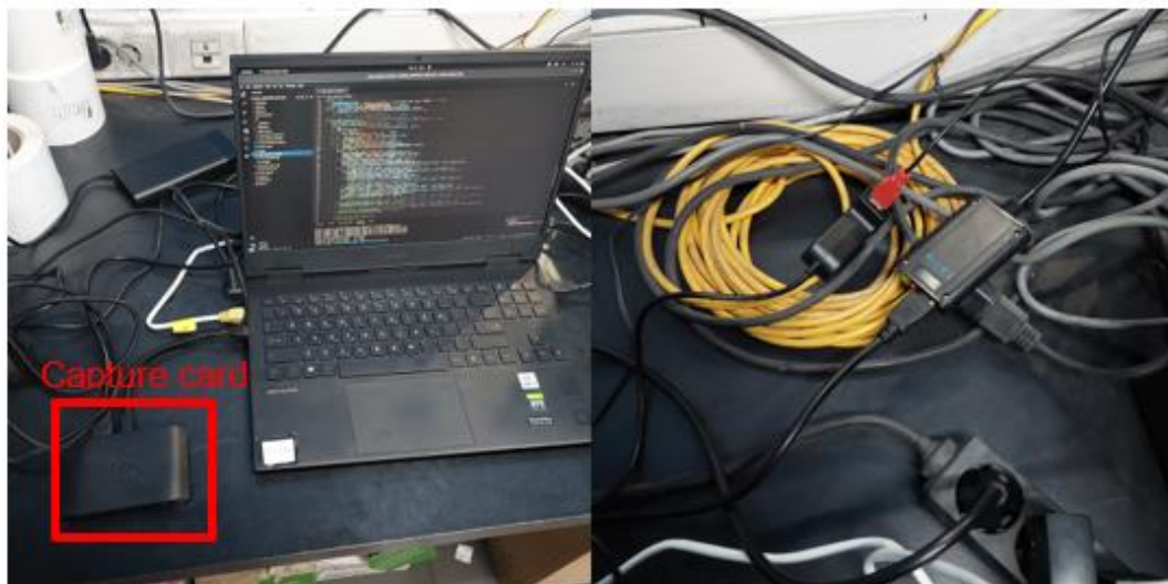
Figure 38: The capture card and the cabling used for monitor mirroring.
