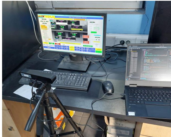
Figure 36: Initial approach recording the screen with a camera.
